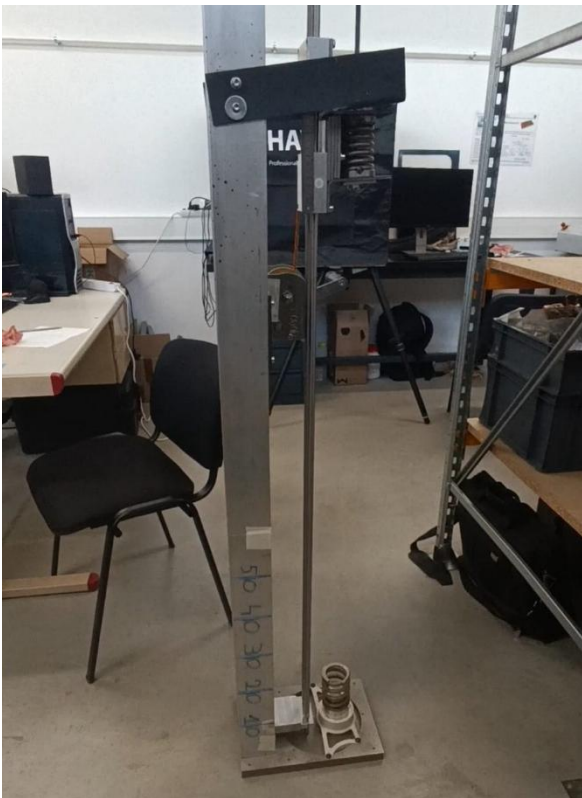
Figure 44: Position ressort mobile, initialement comprimé de 30%
